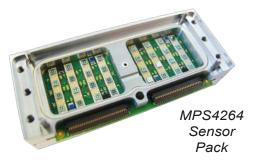
Along with the pressure sensors, all components in the measurement circuit are effected by temperature and drift over time. Scanivalve designed a patented architecture which continuously corrects for these changes over time, while the unit is scanning. This technique of "Dynamic Zero Correction" greatly improves the stability of the entire system over time and temperature. This is accomplished completely "behind the scenes," does not affect performance and requires nothing of the user.
