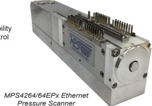
The EPx version still maintains the same robust features that are found in the MPS4264 series scanners. Communication protocols remained unchanged. Precision Time Protocol is available for time correlated data, and scan data can be collected via TCP, FTP, or UDP at scan rates up to 2500Hz\*. A TCU option is available for the MPS/EPx.
