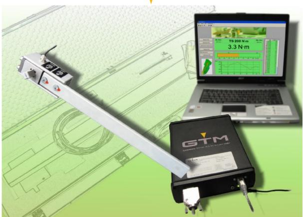
The Torque Transfer Wrench Calibration Set is evidence of conftable and fast inspection of torque wrench kalibration devices. And also for the calibration of torque testing rigs under the effect of a shear force according to DKD-R 3-8
