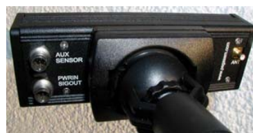
SAT100 rear panel connectors
