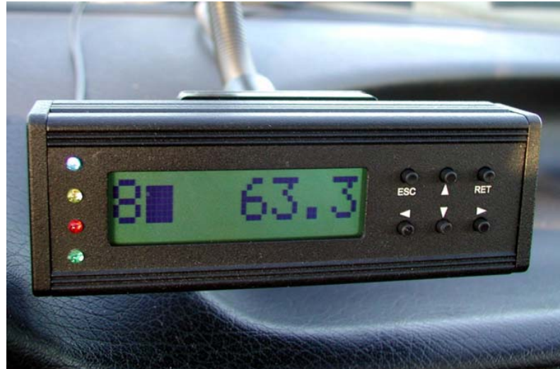
SAT100 receiver with integrated speed display, gooseneck holder and suction cup
